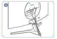
Secure the HOLDER-CABLE to the stand. (HOOK type)
