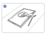
Place the protective Styrofoam (cushion) included in the package on the floor and place the product facing down on the Styrofoam, as shown in the image. If Styrofoam is unavailable, use a thick sitting mat.
