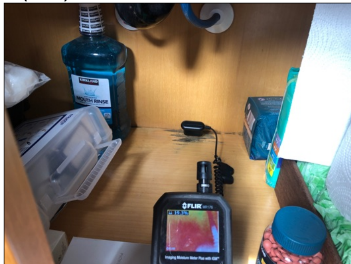
Elevated moisture at right hand sink at master bathroom. (Blue)
